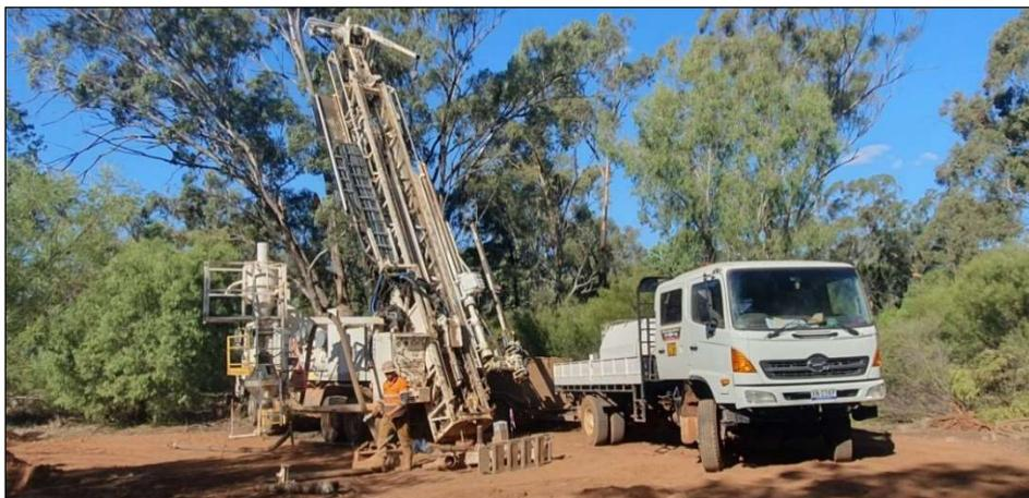
**Figure 1:** Tallebung Tin Project – RC drilling rig onsite at the Tallebung Tin Project.
