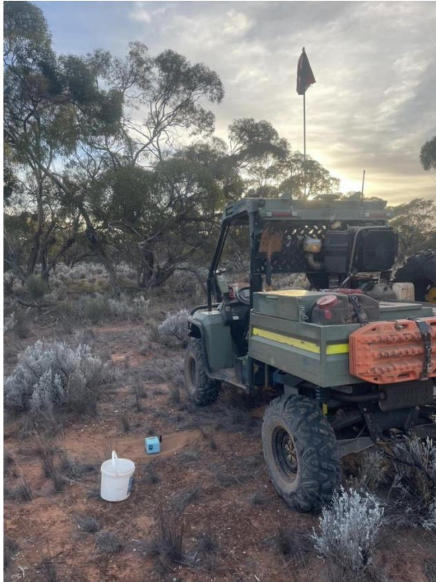
Figure 3: Tromino seismic sensor being positioned at Hector
