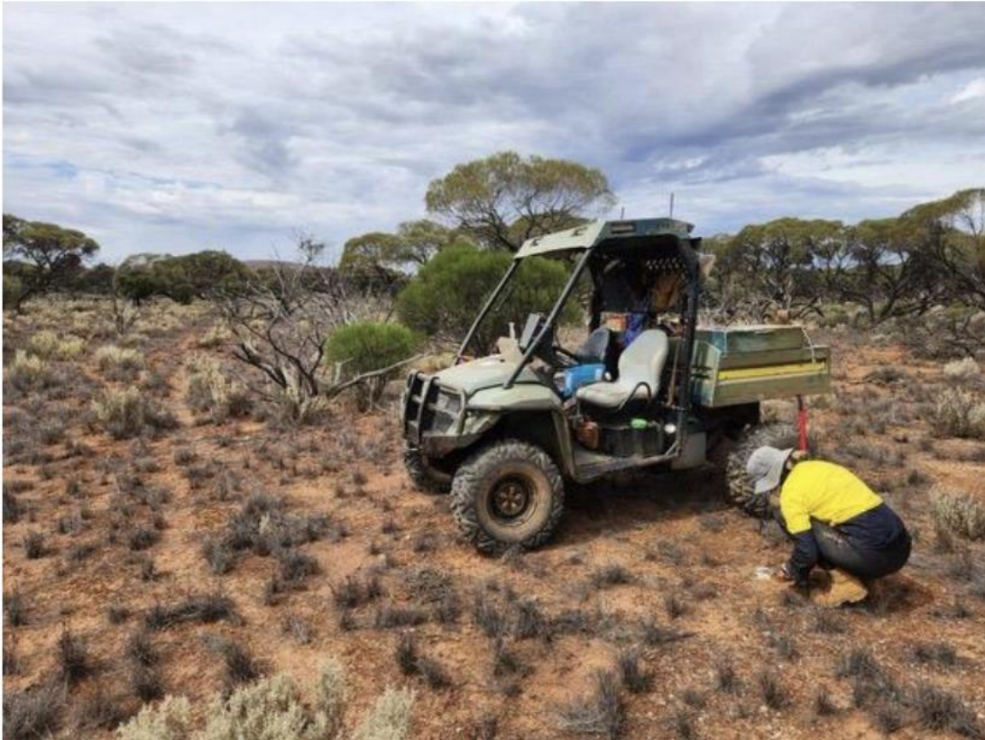
Figure 2: Survey crew laying out ANT seismic sensors at Apollo.
