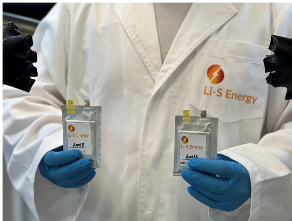
3. Examples of the Phase Two, 2.5Ah lithium sulfur cells tested
