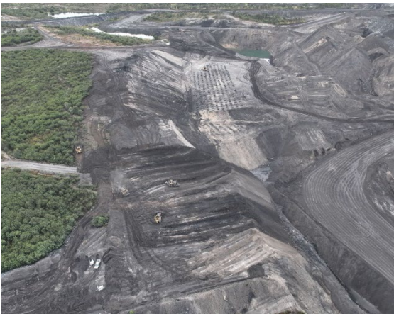
Blair Athol Dozer Push & Blasting Layout
