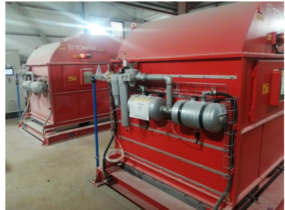
Picture left: The Ore Sorter facilities from outside; Right: the 2 TOMRA XRT Sorters at Barruecopardo
