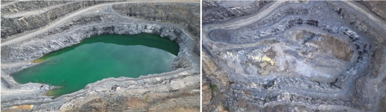
Above Left: The Andy White Open Pit as of the 1st of January 2024, Right: the pit dewatered on 22 nd February 2024
