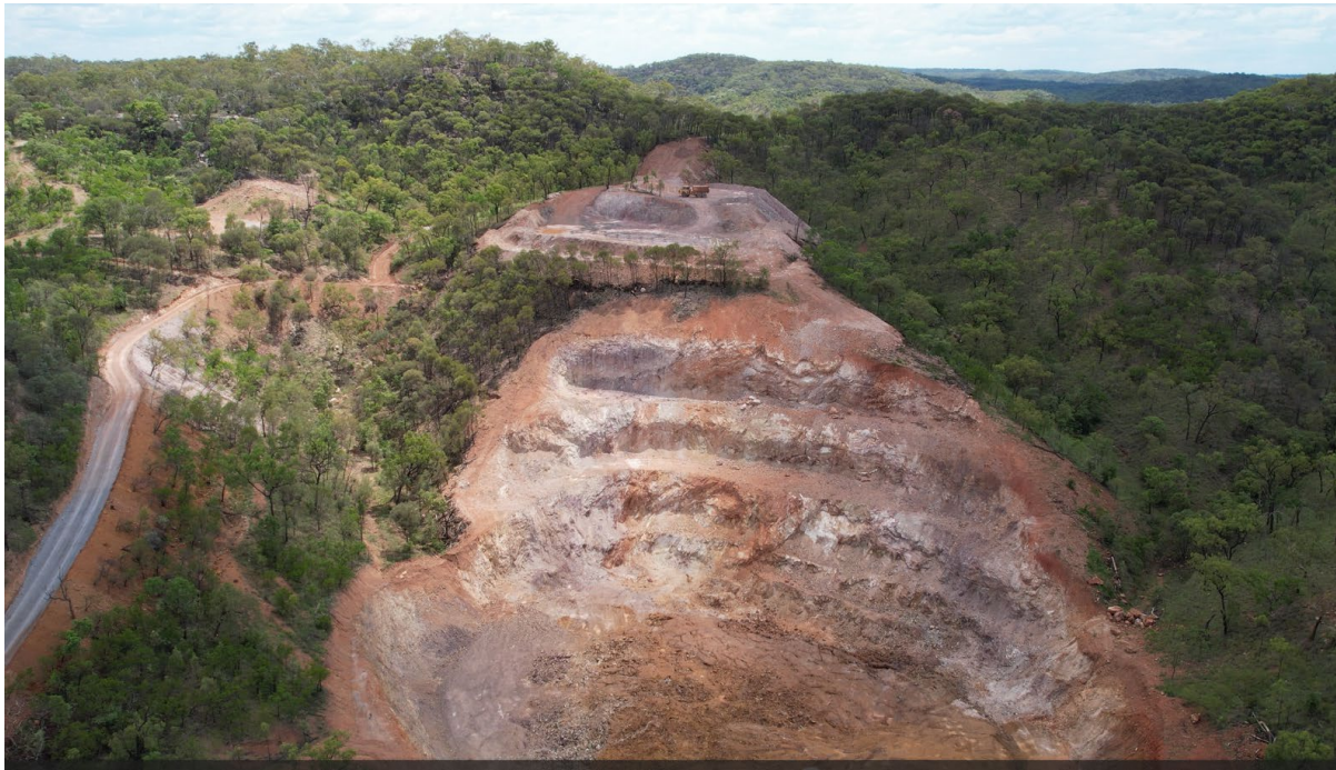
Sherwood West Pit 1 – mining the up dip extension of structure outcropping at top of hill
