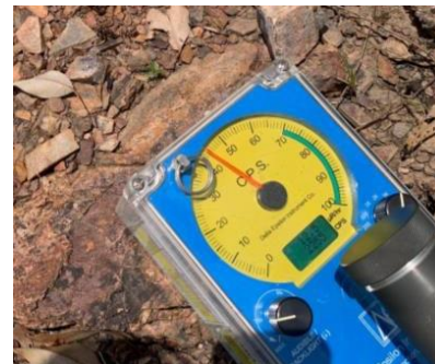
Elevated radioactivity from scintillometer (2,255cps)
