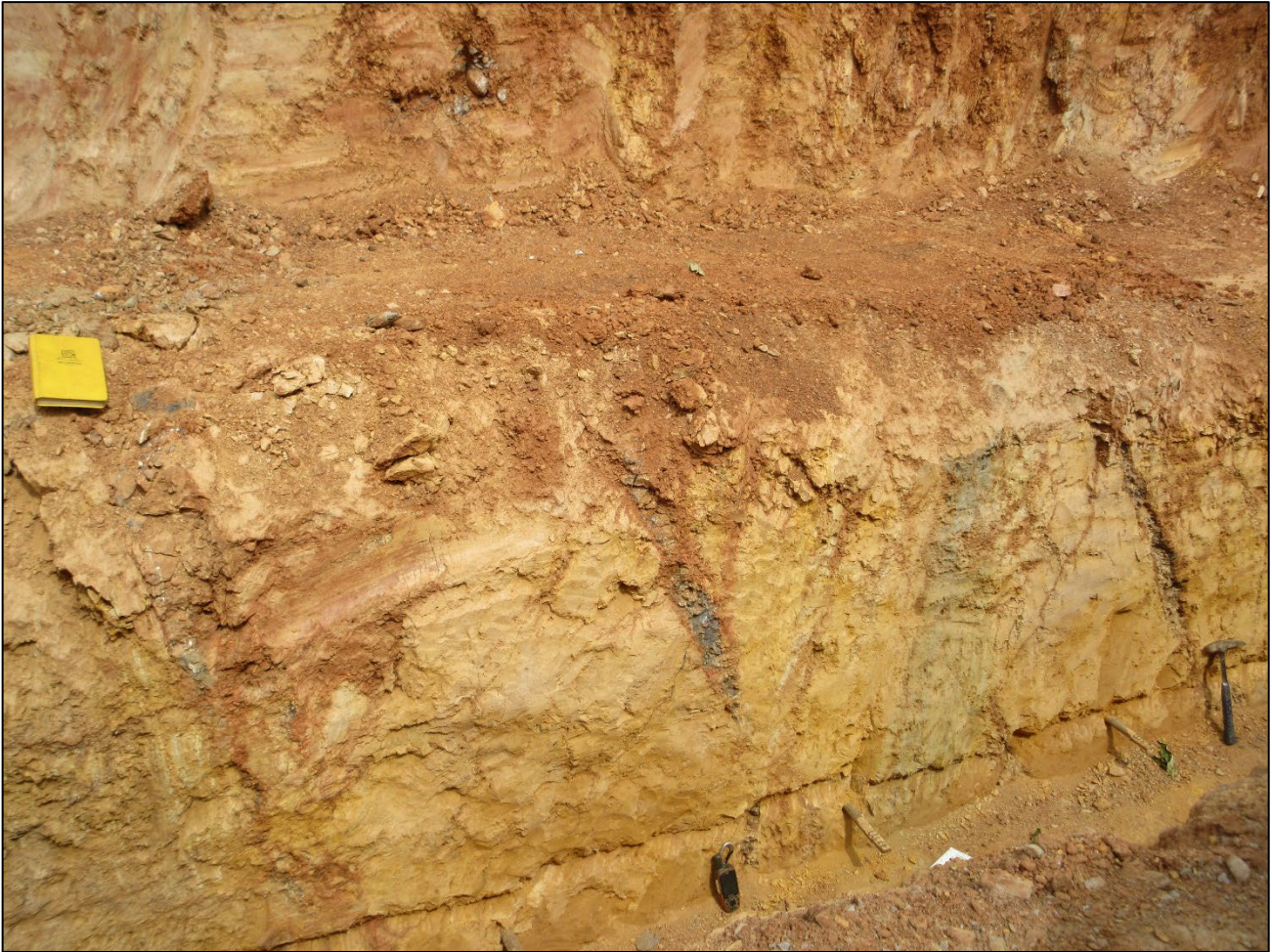
Figure 3: Trench NATR012 at Central Zone – note the greyish quartz veins as well as stockwork of reddish-brown oxidized quartz stringers throughout the host rock
