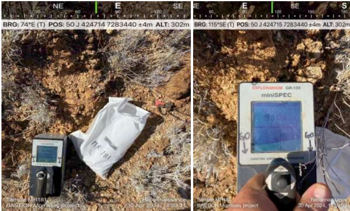
Figure 4: High spectrometer measurement (5885 to 9405 cps) at sample MR181 site (424714E, 7283440N, UTM Zone 50) in the west of the property. No uranium minerals noted.
