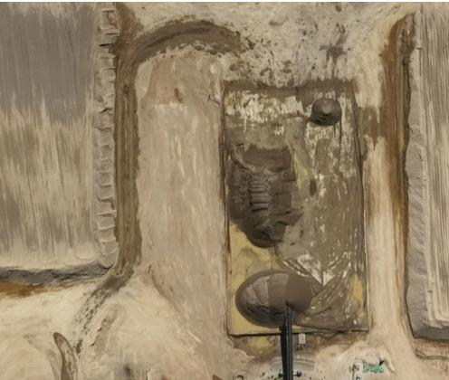
**Image 1:** Wet concentrate overflow storage pad. Used for >12% moisture for free draining of water. **Status:** 17<sup>th</sup> May, Complete.
