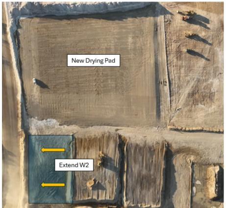
**Image 2:** Northern drying pads. Used for <12% moisture for final solar drying. **Status:** 19<sup>th</sup> May, Complete
