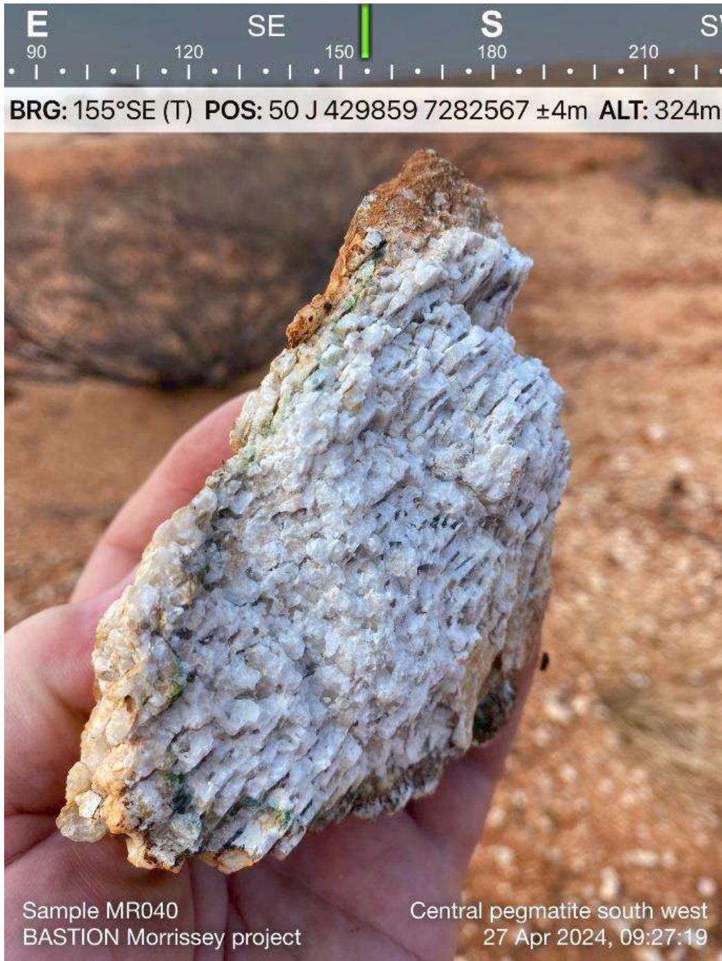
Figure 1 - Pegmatite sample MR040 exhibiting graphic textures, to be assayed for lithium. 429859E/7282567N UTM Z50. See coordinate captured at the top of the photograph. (approximately 25% quartz within feldspar in primary concordant texture);
