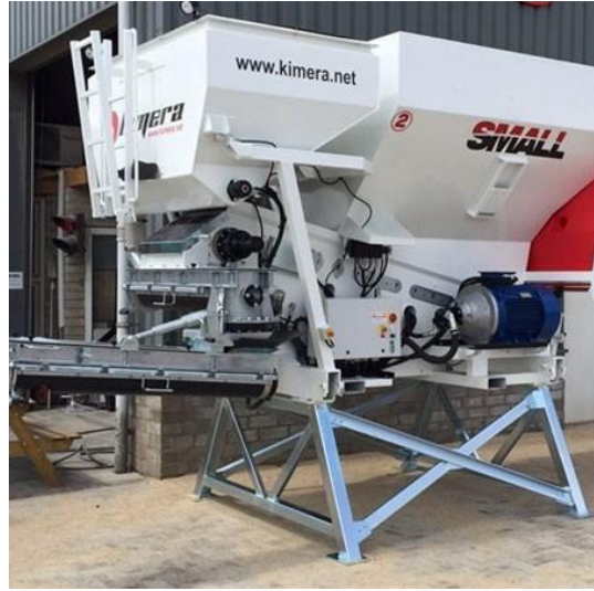
Figure 22: Small mobile concrete batch plant
