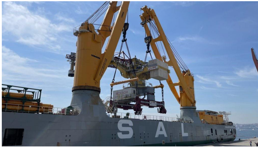
Figure 37: HLS lifting a fully assembled shiploader
