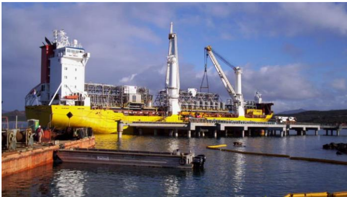
Figure 3031: HLS transporting prefabricated modules
