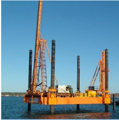
Figure 2021: SEMP used to install mooring piles.
