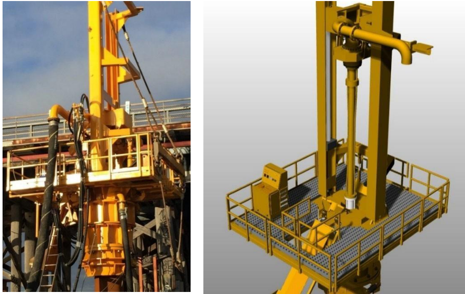
Figure 28: Pile top drill rig used for DDD pile installation
