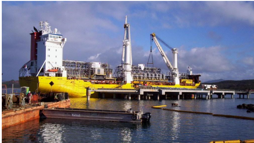
Figure 31: HLS transporting prefabricated modules
