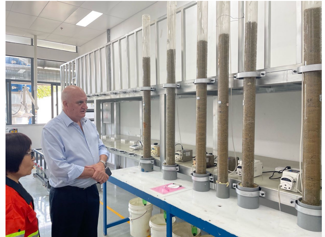
Oxide Column Leach at Zijin Research Labs
