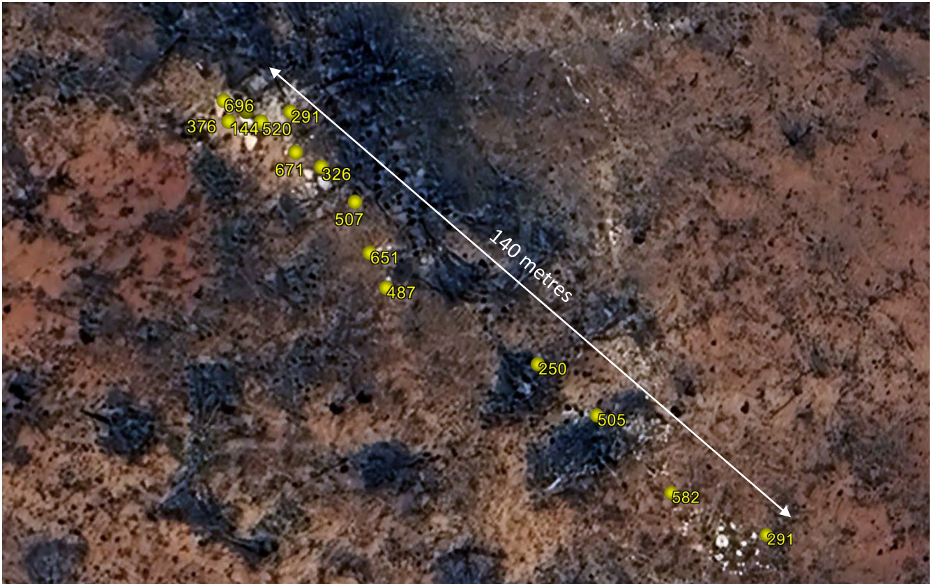
Figure 1. Image of outcropping pegmatite (white) with rock chip locations and Li 2 O assays results (yellow).
