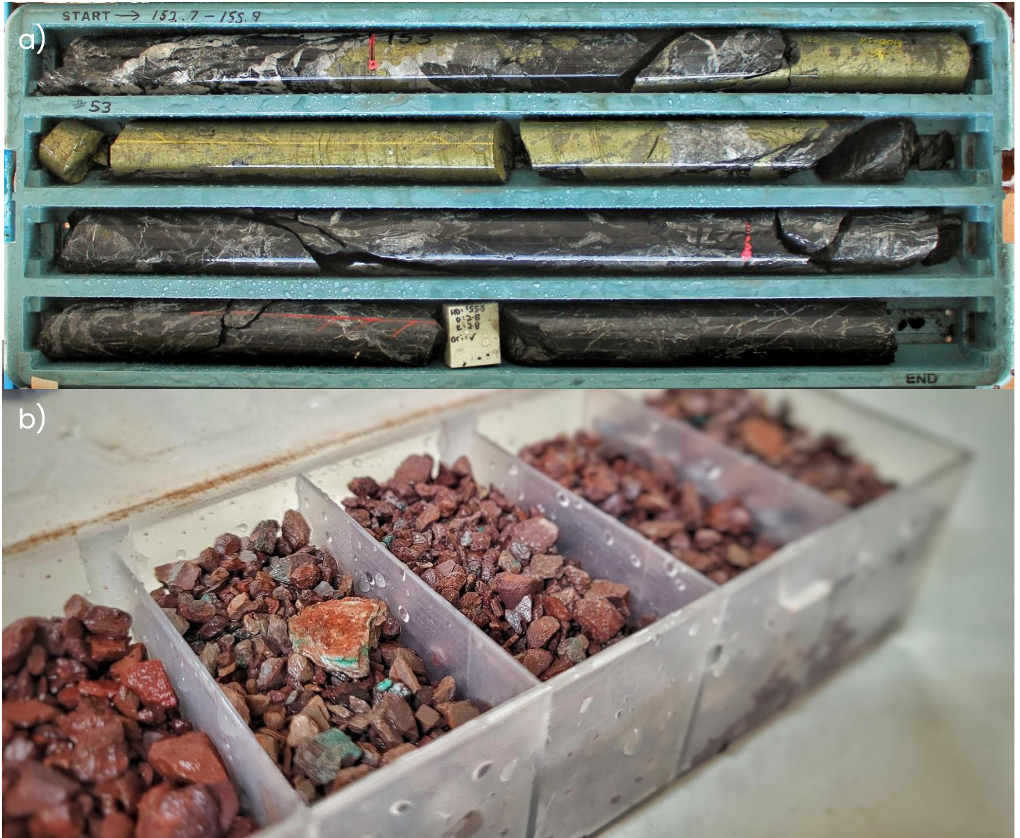
Figure 4: Selected core and chip photos of Cu mineralisation intercepted in the 2023 Flying Horse Drilling Program. a) A lens of massive chalcopyrite hosted within faulted/ brecciated weakly carbonaceous shales (MTKD019, 152.7 - 155.9m). b) Chip tray photo showing Cu oxide mineralisation (malachite and chrysocolla) hosted in ferruginous saprock (MTKC0662, 36-40m).
