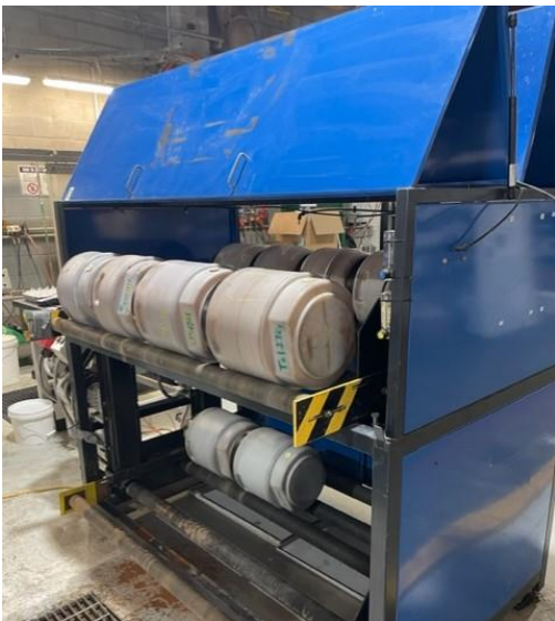
[Figure 2] Sybella Project: Intermittent bottle roll leach tests or IBRT (left), example of column leach tests (right)
