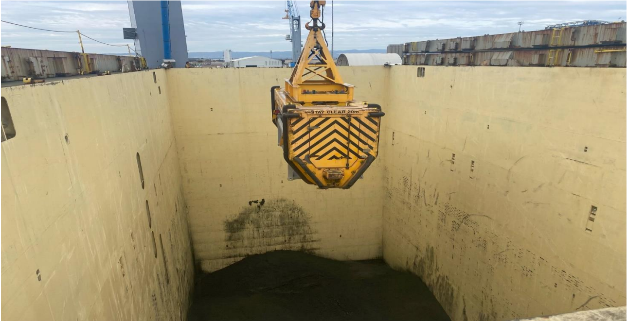
Figure 2 Concentrate Tipped into Vessel's Hold Via Rotainer System
