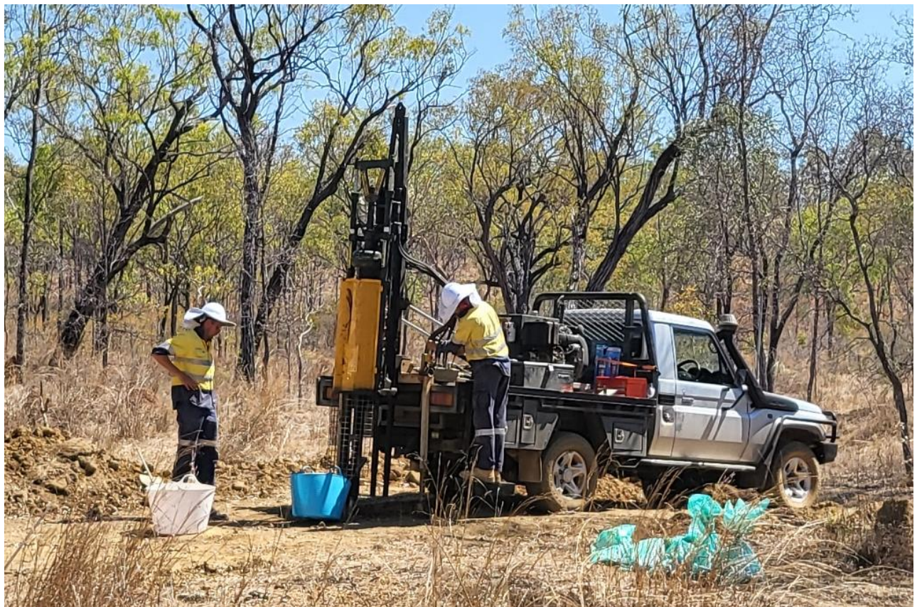
Figure 1: Ark's auger rig drilling to around 4m depth in Sandy Mitchell mineral sands.
