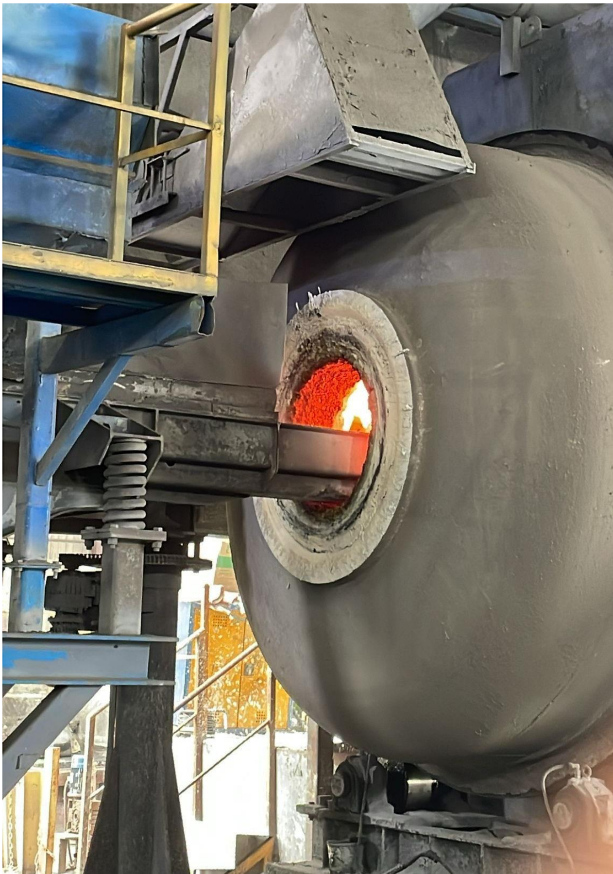
Figure 2 – Iberian Smelting's Rotary furnace, feeding hopper and exhaust hood
