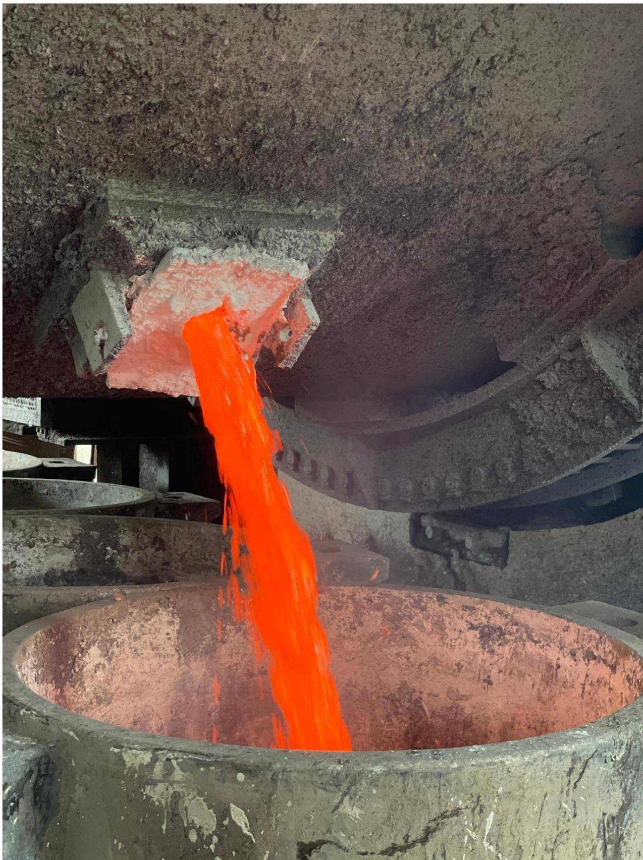
Figure 3 – Tin metal pouring out of the rotary furnace's spout into pots at the Robledallano smelter
