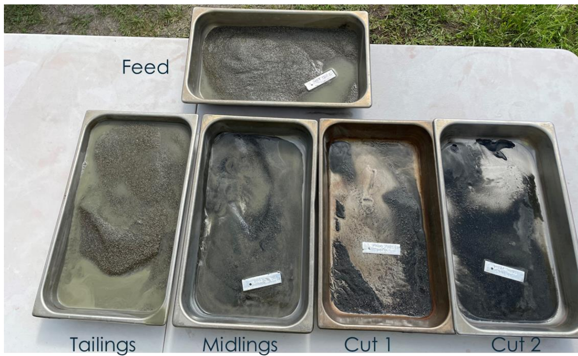
Figure 3 – Separation Products from Rougher Spiral Processing
