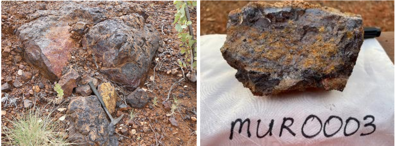
Figure 3: Iron rich rocks from Mt Ulo, LHS outcrop near UR01; RHS sample from cross structure MUR0003: 1,790ppm Cu, 235ppm Co (Red Fox sampling)
