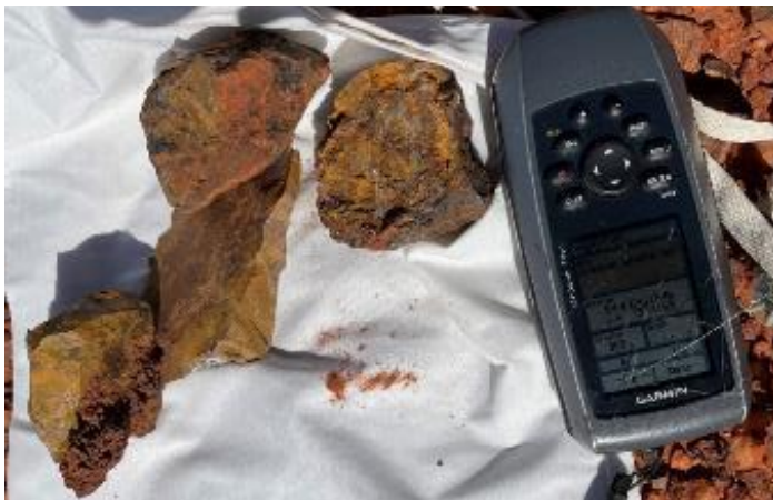
Figure 7: Jasper Ridge West rock sample JRR0005 - 0.26g/t gold, 338ppm cobalt, 3,410ppm copper
