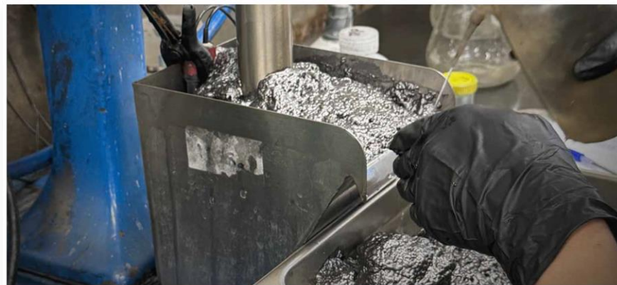
Figure 1. 94% TGC concentrate produced from the Lacroma Deposit
