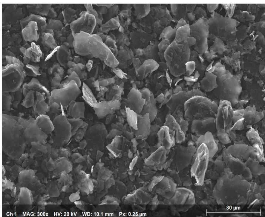
Figure 2. Scanning electron microscope image of the Lacroma graphite concentrate showing fine (-75 micron) particle size suitable for PSG production
