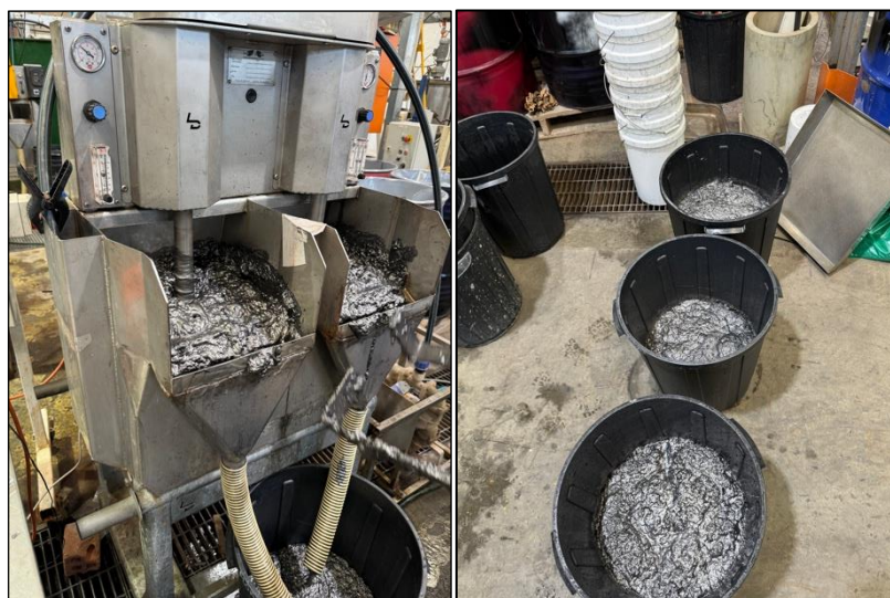
Figure 1. Bulk scale flotation cell (left) with Lacroma graphite flotation concentrate (right)
