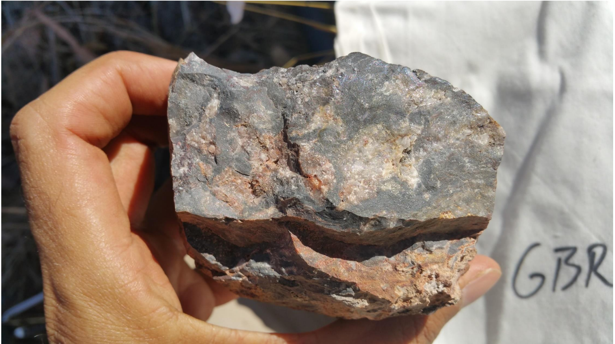
Figure 6. GBR047. Vein quartz with medium to coarse-grained textures brecciated infilled with fine-grained low-temperature silica - 16,061ppm TREO
