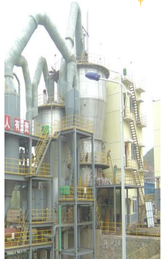
BGRIMM 200tpd Two-Stage Fluidized-Bed Roaster
