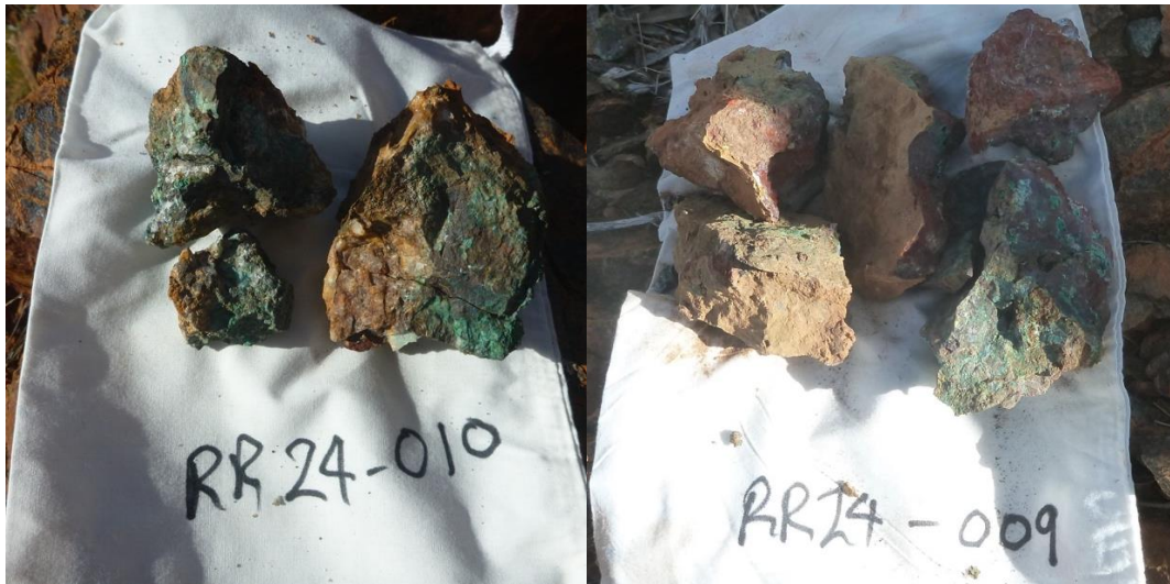
Figure 5. Rock chip sample locations at the Scimitar prospect containing green malachite (copper) mineralisation. RR24-010 (right) assayed 3.3 g/t Au and RR24-090 assayed 1.0 g/t Au.
