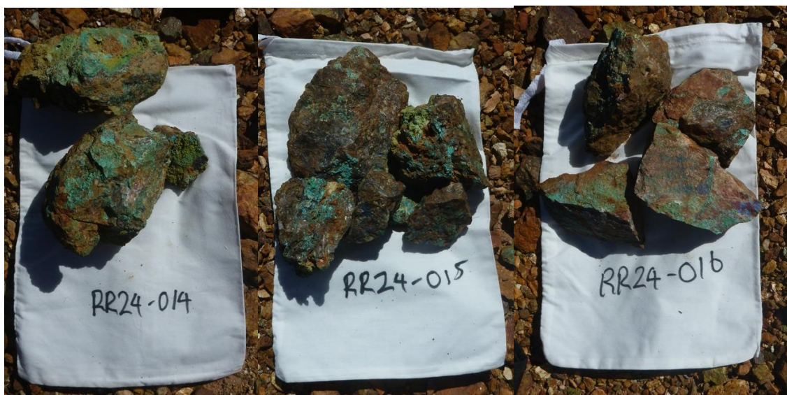
Figure 6. Copper mineralisation at the Reward copper mine, containing green malachite and chrysocolla and blue azurite mineralisation. Sample RR24-014 (left) assayed 0.61 g/t Au, sample RR24-015 (centre) assayed 1.0 g/t Au and sample RR24-016 (right) assayed 1.0 g/t Au.
