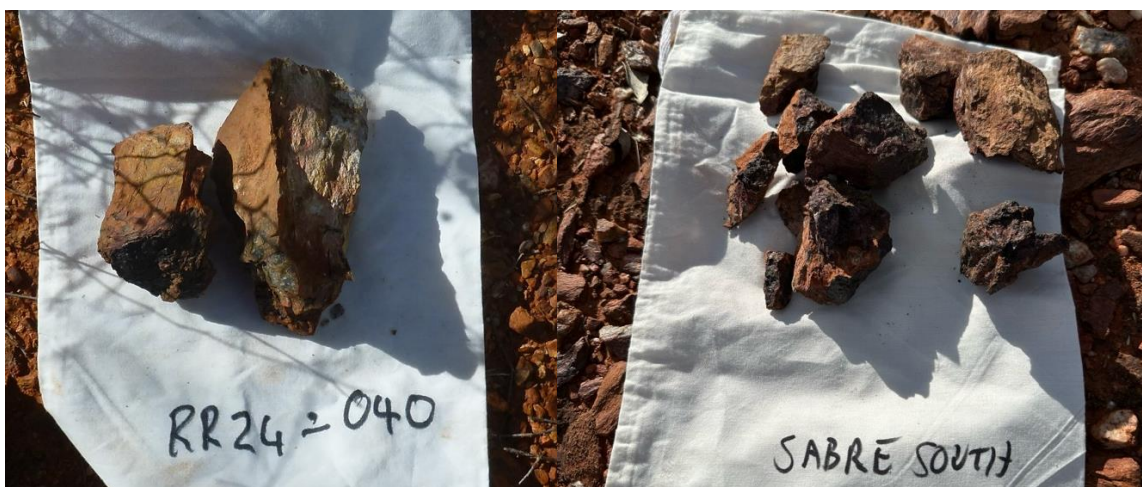
Figure 3. Sample RR24-040 on the left assayed 182 g/t Au and sample RR24-044 on the right assayed 4.1 g/t Au
