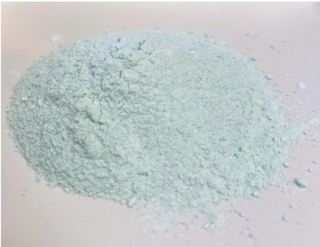
[Figure 1] Sybella Project: Maiden mixed rare earth carbonate product (8.2g dry weight) following innovative impurity removal trials on pH 1.3-1.7 Pregnant Leach Solution (PLS) derived from the Phase 2 bottle roll leaches.
