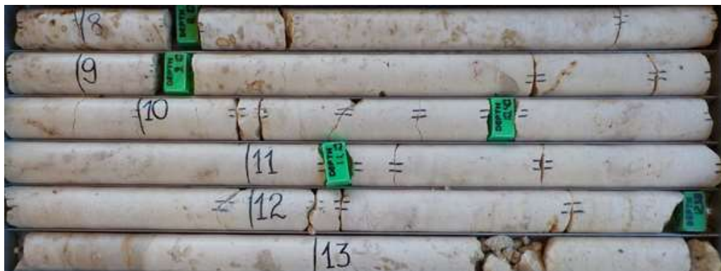
Fig 5 - Soalara Limestone - High purity @ 97% Calcium Carbonate, CaCO 3 - from 8m depth
