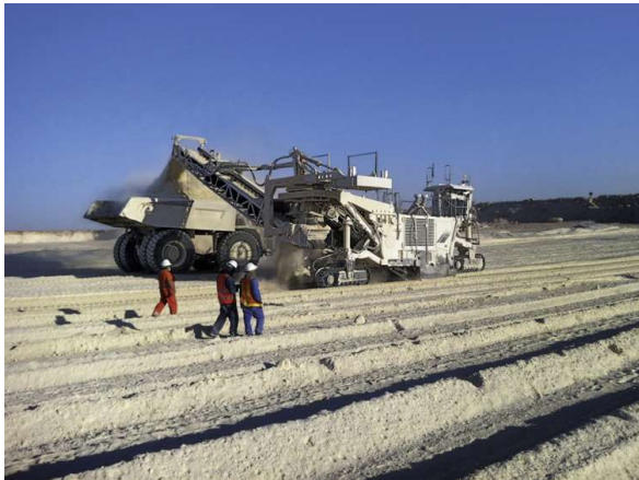
Fig 3 – Example Surface Miner – Limestone row cutting at variable heights Fig 4 – High purity Soalara Limestone core
