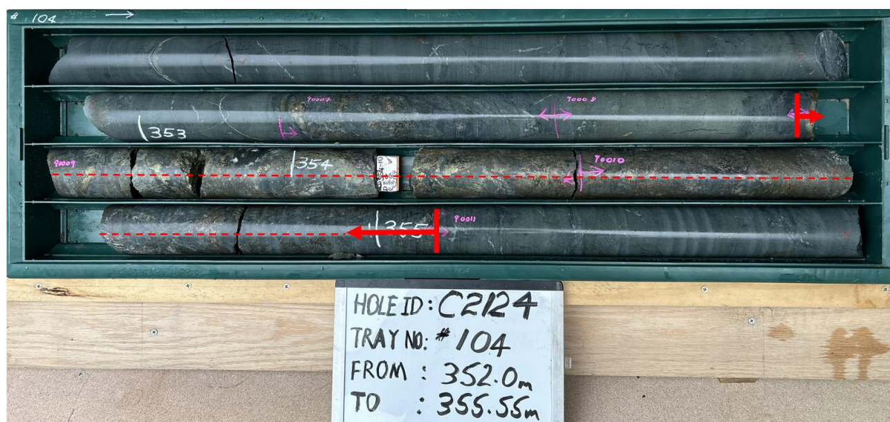
Figure 3. Drill hole C2124 depicting the tin-copper mineralisation from 353.7m to 355.1m.
