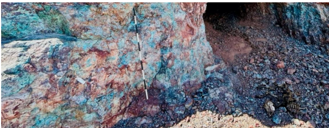
Figure 1 Channel Sample taken Across Copper Staining Mine Entrance
