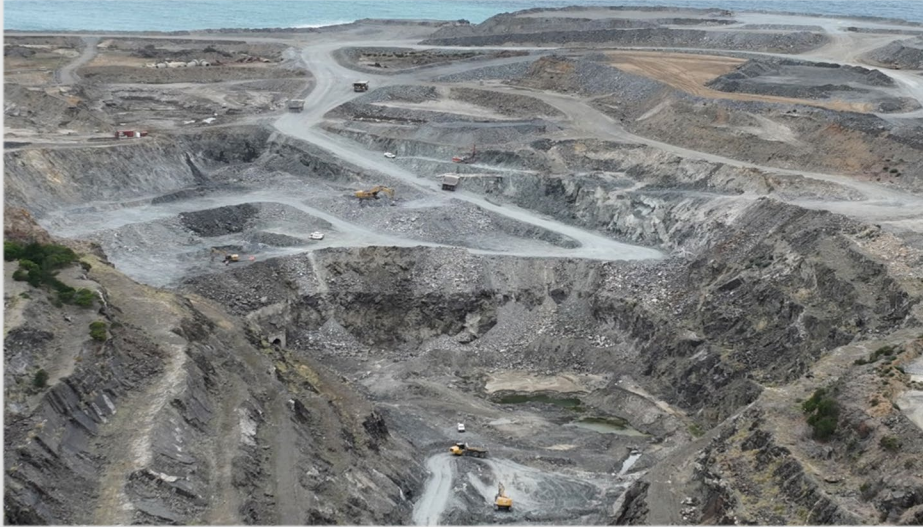
Dolphin Tungsten Mine – Stage 1 Mining High Grade Ore (0.91% WO 3 )
