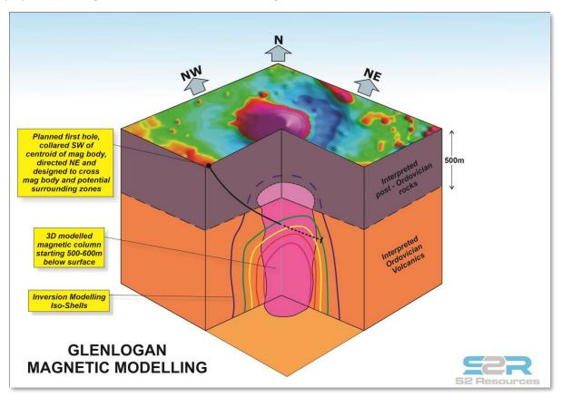
Figure 2: Schematic cutaway block diagram showing the modelled magnetic column in 3D and where the first hole is planned to test it
