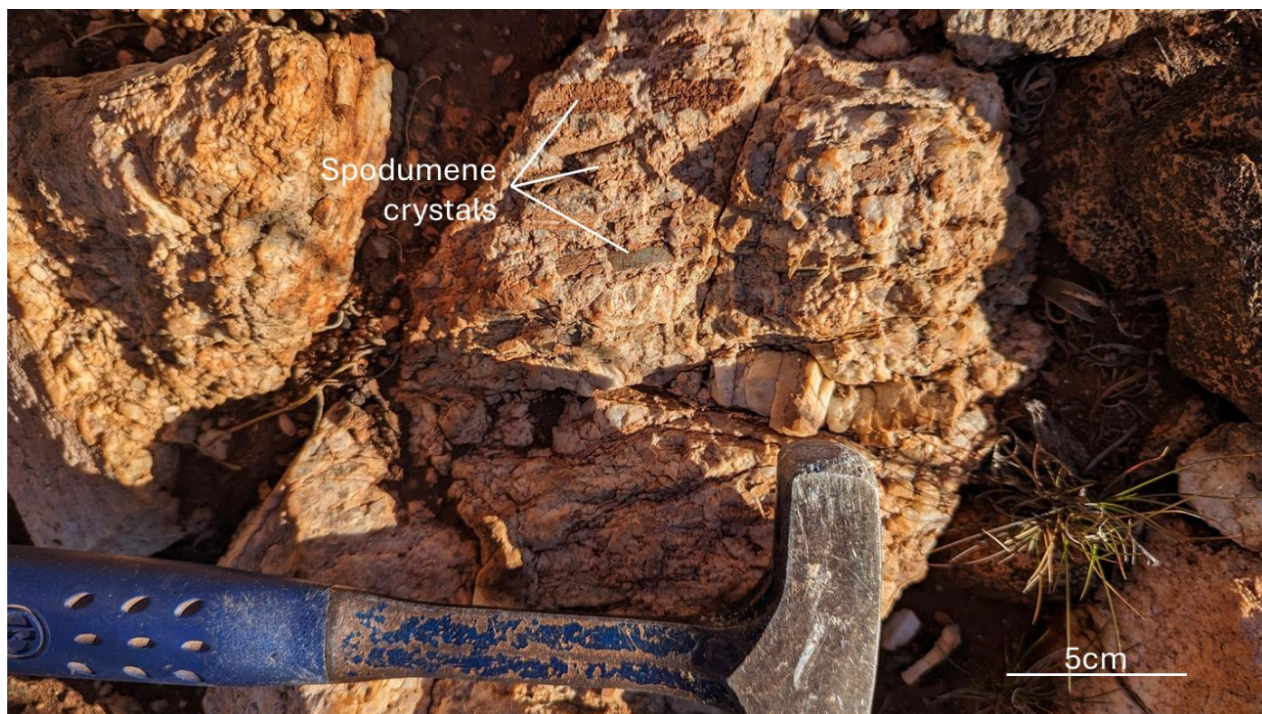
Figure 4 - Larkinville pegmatite outcrop sample with weathered spodumene crystals grading 1.3% \text{Li}_2\text{O} (SMX00958).
