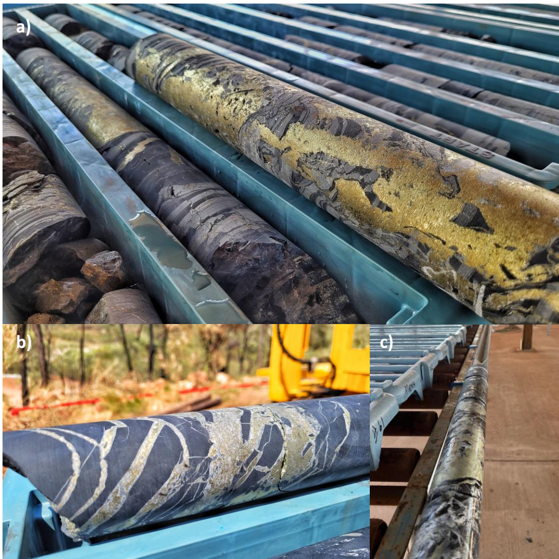
Figure 4: Selected core photos of Cu mineralisation intercepted at Lady Colleen. a) Semi-massive chalcopyrite breccia fill typical of mineralisation associated with the Spinifex Fault (MTKD017, 223m). b) Crackle-breccia filled chalcopyrite-dolomite associated with the carbonaceous shale unit (MTKD017, 274m). c) Narrow, but strong chalcopyrite mineralisation intercepted in MTKD014 (189m).
