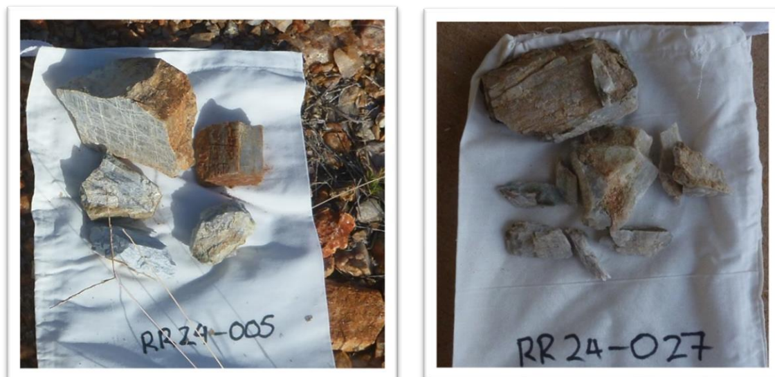
Figure 1. Rock chip samples of QXRD confirmed spodumene from the GMF Pegmatite
