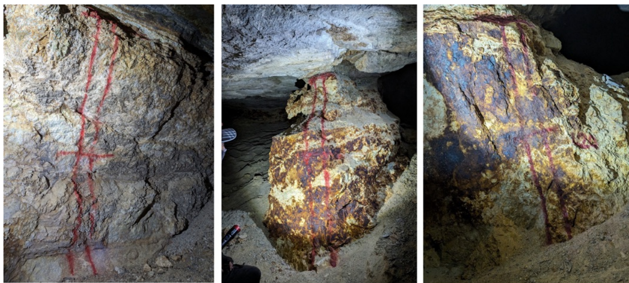
Figure 8 Inside El Refugio workings, Left to right – sample line 12 (L12) - 1.5m @ 9.33 g/t Au, 173 g/t Ag, sample line 28 (L28) - 2.0m @ 6.91 g/t Au, 148 g/t Ag, and sample line 30 (L30) - 2.0m @ 39.2 g/t Au, 401 g/t Ag.
