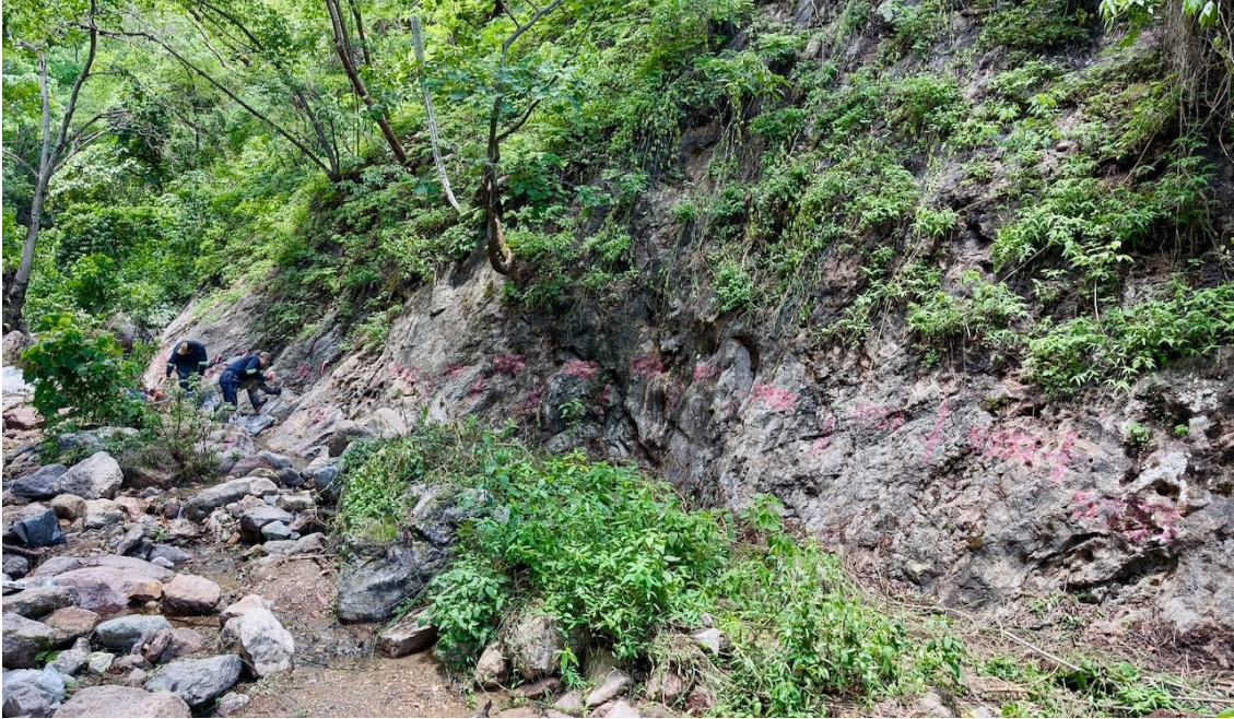
Figure 5 Channel sampling across vein at Copalquin Creek – Zaragoza area.
