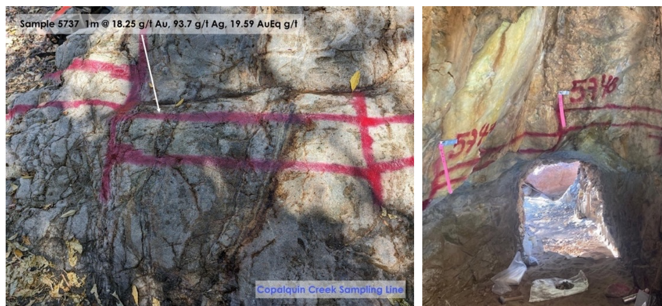
Figure 10 Left: Mineralised structure in the Copalquin Creek important for the overall district geologic model. Right: Inside the historic Copalquin mine showing diamond saw channel sample.
