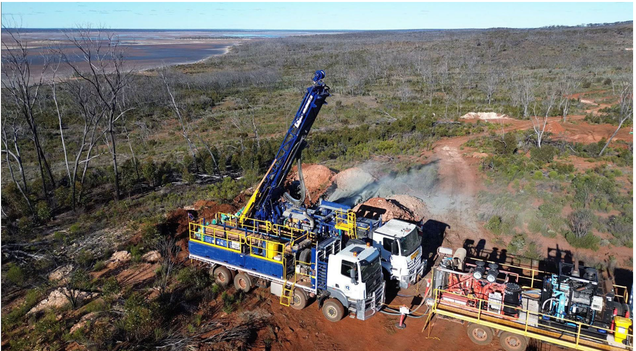
Figure 1. RC rig drilling lithium zones at the Maggie Hays Hill Project
