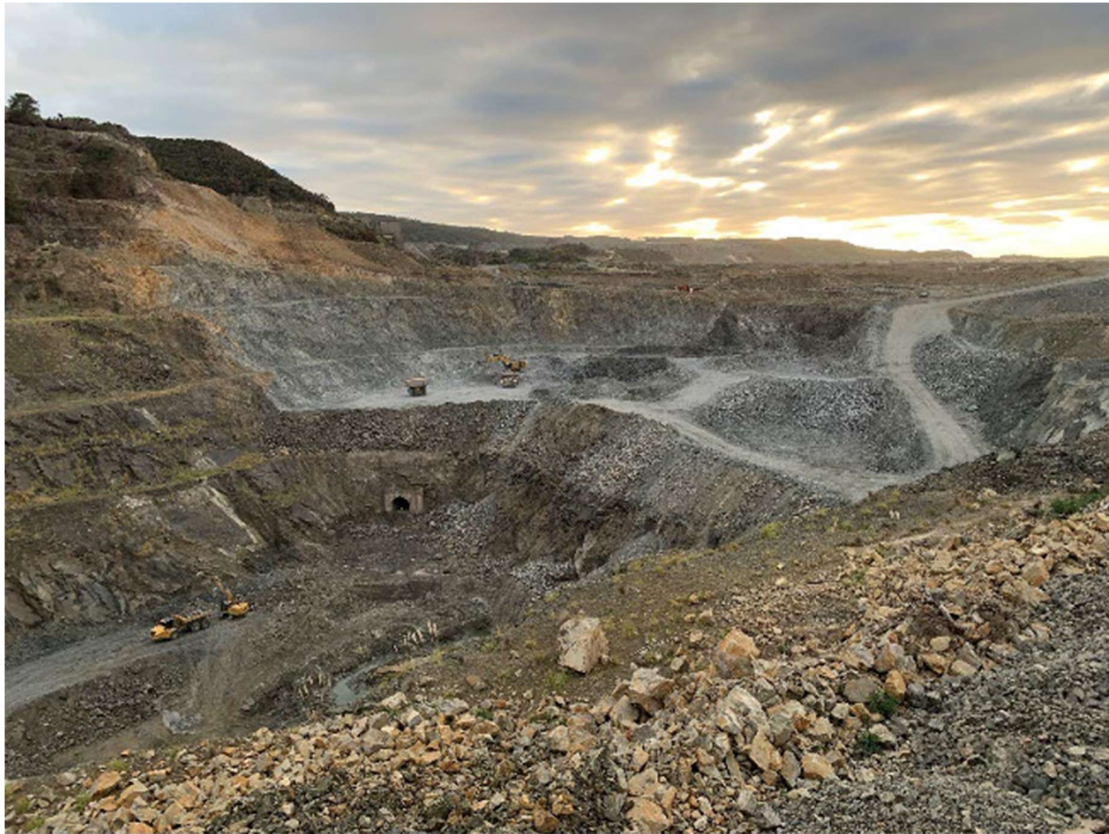
Figure 3 - Dolphin Open Cut Stage 1 Bench Development at RL-30m, above high-grade C-lens - May 2024
