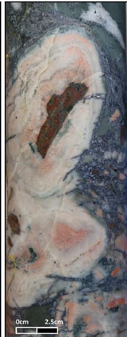
ML001 at 152.7m - Quartz-galena-sphalerite-adularia-chalcedony cockade breccia.
