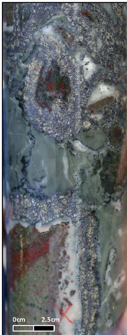
ML001 at 149.8m - Quartz-galena-sphalerite-chalcopryrite-adularia-chalcedony cockade breccia.
