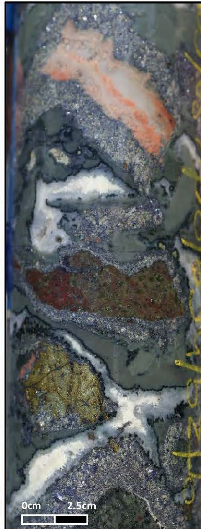
ML001 at 151m - Quartz-galena-sphalerite-chalcopryrite-adularia-chalcedony cockade breccia.
