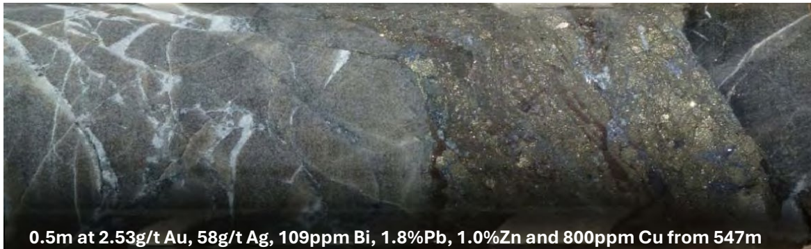
Mineralisation an altered breccia zone with sphalerite (brown), galena (silver) and pyrite (gold colour). CUT A DO1 core 547m
