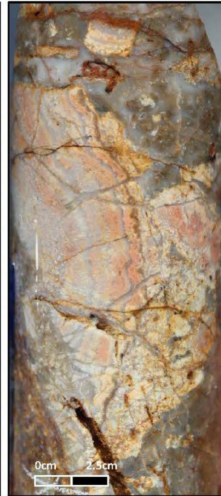
BK001 at 29.8m – chalcedony- quartz-adularia breccia with chalcedony-quartz matrix
