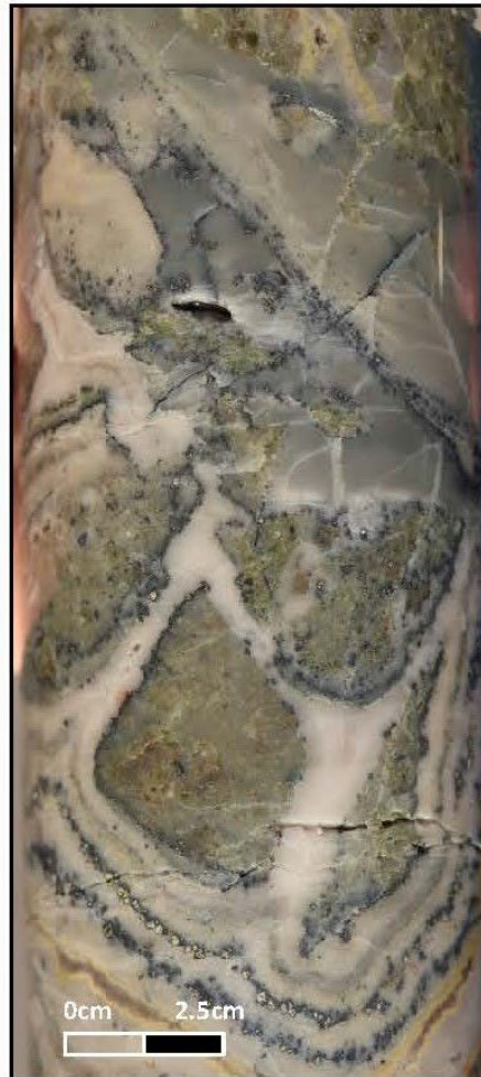
BK002 at 109.35m – chalcedony-quartz-adularia- sphalerite-galena cockade breccia
