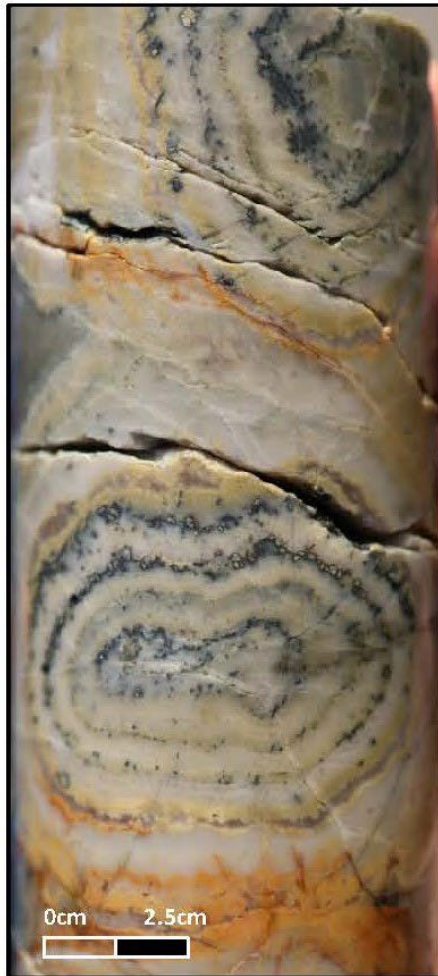
BK002 at 109.35m – chalcedony-quartz-adularia- sphalerite-galena cockade breccia
