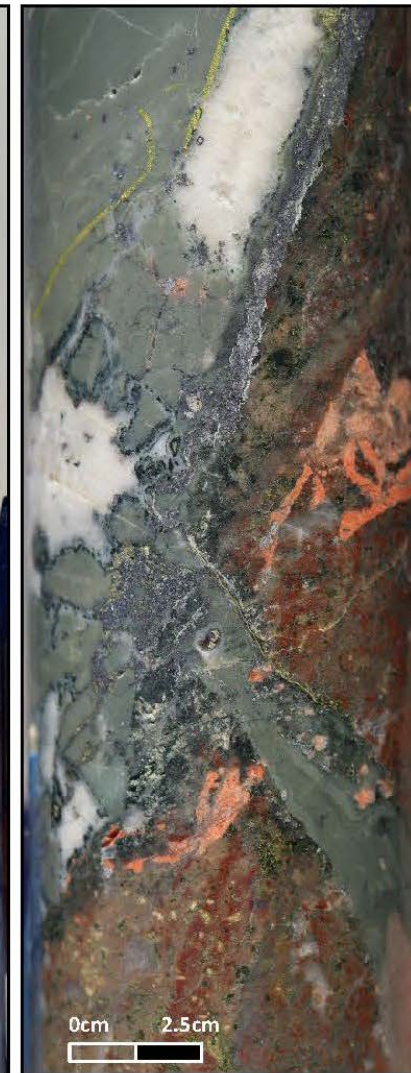
ML001 at 154.8m - Quartz-galena-sphalerite-adularia breccia with quartz-chalcedony matrix.
