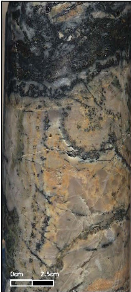
BK002 at 108.1m – chalcedony-quartz-adularia- sphalerite-galena-pyrite cockade breccia
