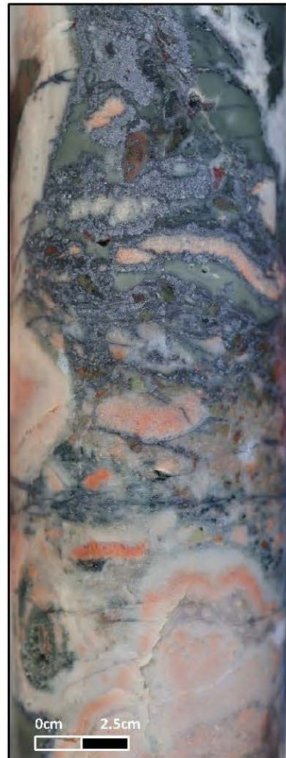
ML001 at 152.7m - Quartz-galena-sphalerite-adularia-chalcedony cockade breccia.
