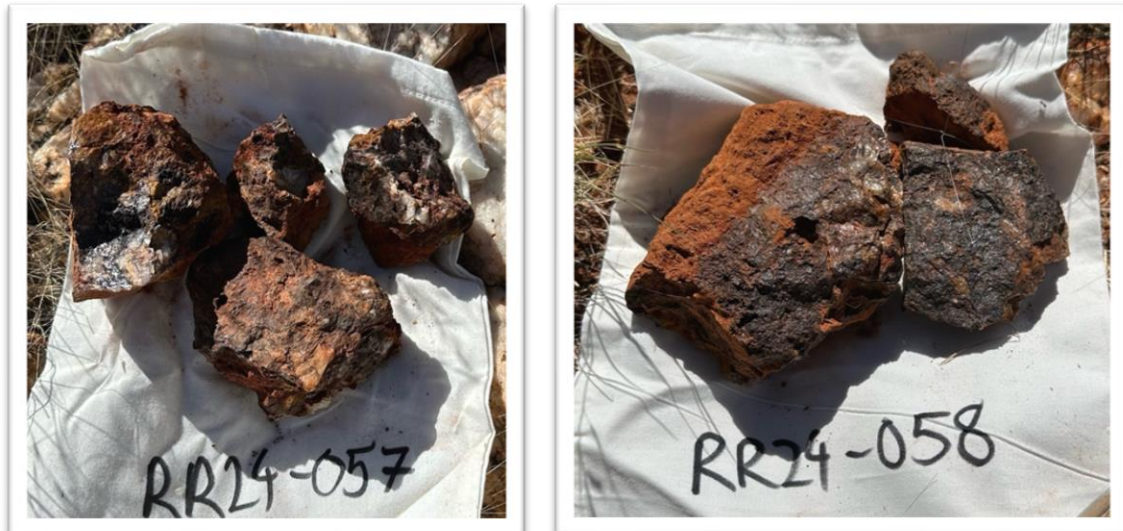
Figure 5. Rock chip samples of gossanous quartz veins from over the EM anomaly at the Scimitar Copper-Gold prospect
