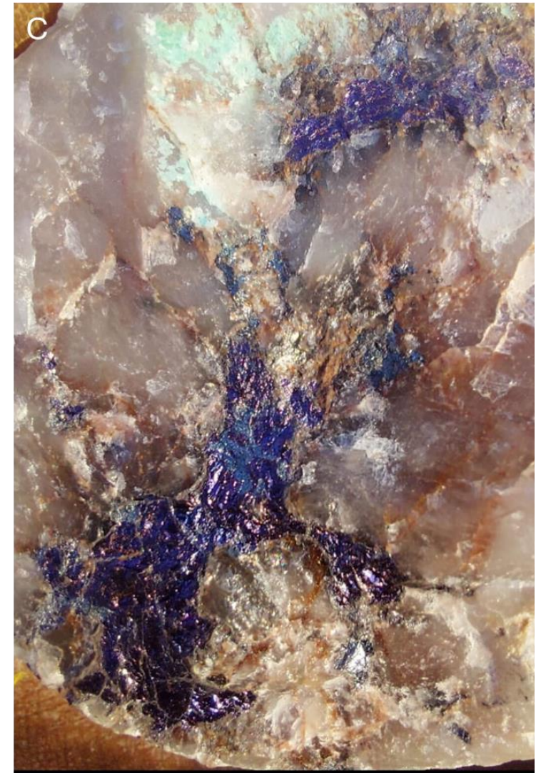
Figure 2. Vein hosted copper mineralisation. (A) chalcopyrite and (B) chalcocite mineralisation from drill hole OCP11. (C) and (D) bornite mineralisation from OCP09, all core is HQ size (63.5mm diameter).
