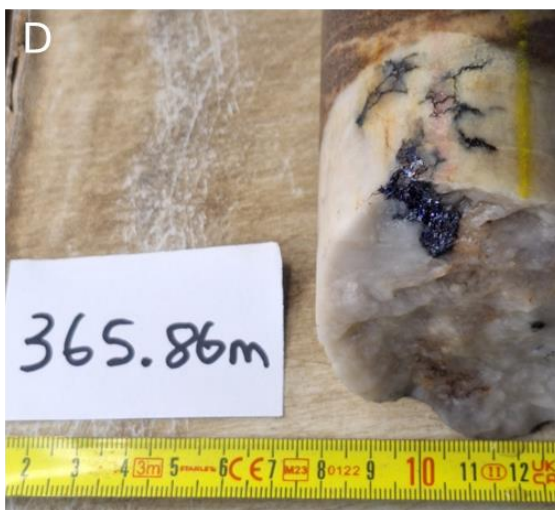
Figure 2. Vein hosted copper mineralisation. (A) chalcopyrite and (B) chalcocite mineralisation from drill hole OCP11. (C) and (D) bornite mineralisation from OCP09, all core is HQ size (63.5mm diameter).
