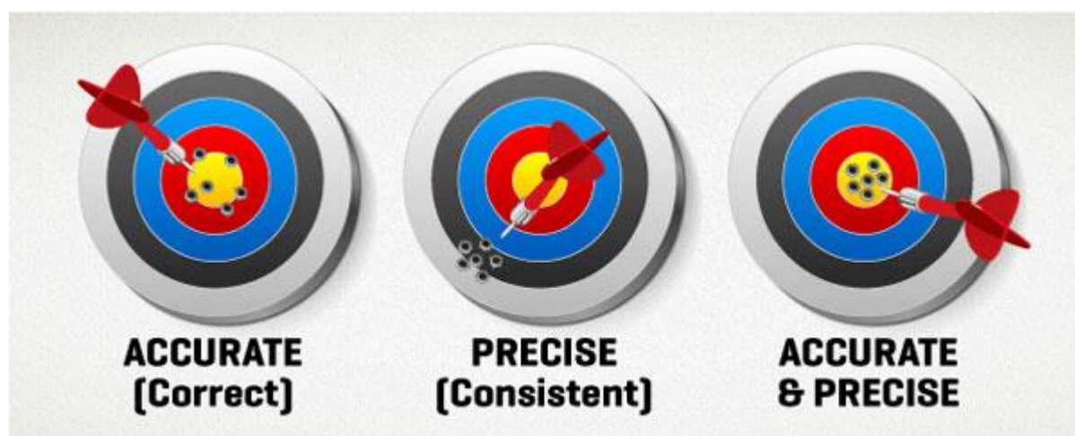
Figure 5.12 – Accuracy vs Precision
