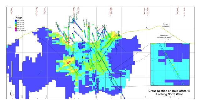
Figure 4: Section A-A' showing drilling grades vs block model grades
