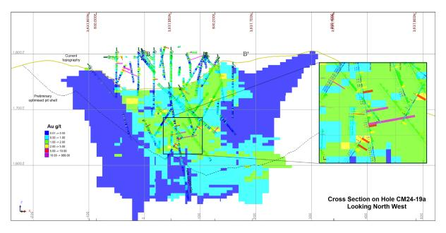
Figure 5: Section B-B' showing drilling grades vs block model grades
