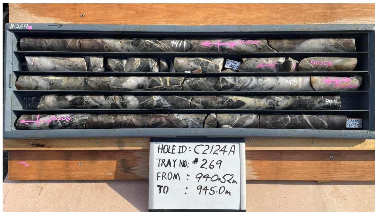
Figure 4. Mineralised quartz/sediment breccia within drill hole C2124A from 940.5 to 945.0m
