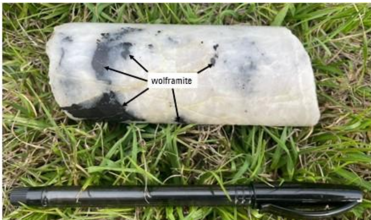
Figure 2. Close-up image of NQ diameter drill core from C2124A from 887.9-888.0m (Figure 3) depicting coarse grained wolframite within a steeply dipping cross-cutting quartz vein.
