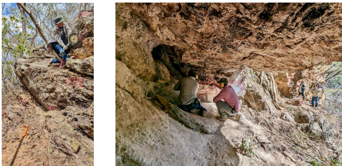
Figure 3 Cutting a channel sample in large outcrop at El Cometa.
