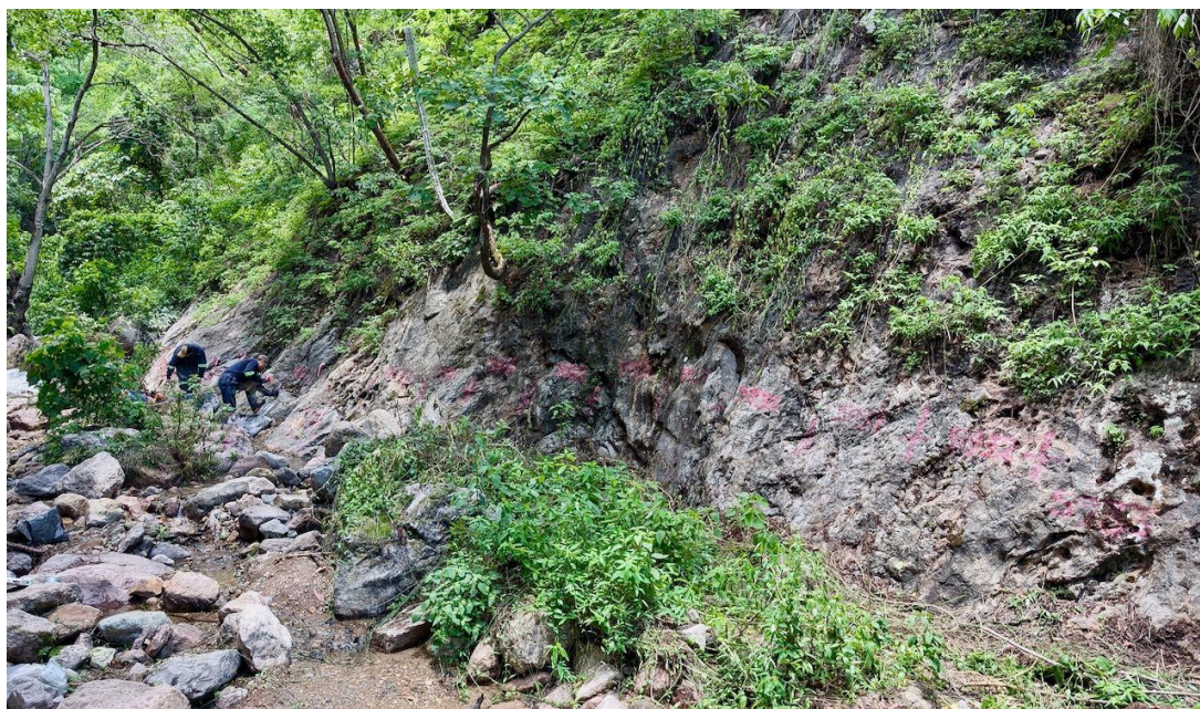
Figure 4 Channel sampling across vein at Copalquin Creek – Zaragoza area.
