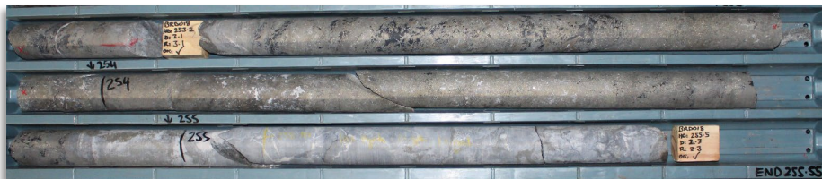
BRD018 , massive sulphide mineralisation (253.0-255.5m)
