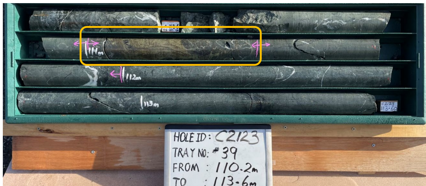
Figure 10. Drill hole C2123, with the orange box indicating the semi-massive copper sulphide mineralisation from 111.0m – 111.45m
