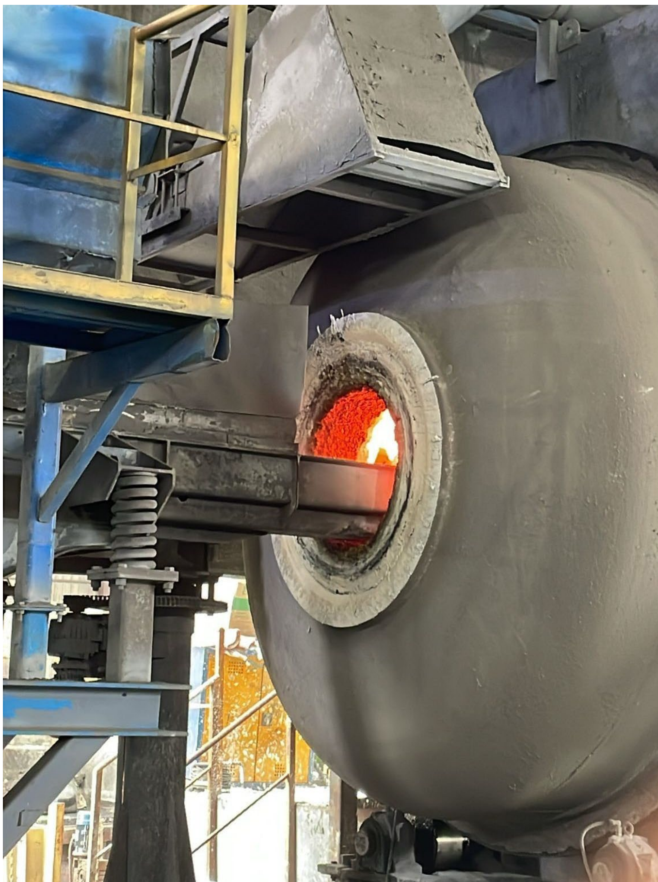
Figure 6. Iberian Smelting's Rotary furnace, feeding hopper and exhaust hood
