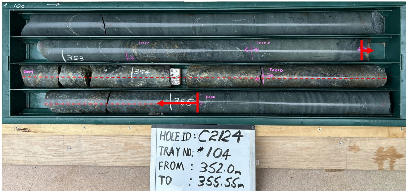
Figure 12. Drill hole C2124 depicting the tin-copper mineralisation from 353.7m to 355.1m
