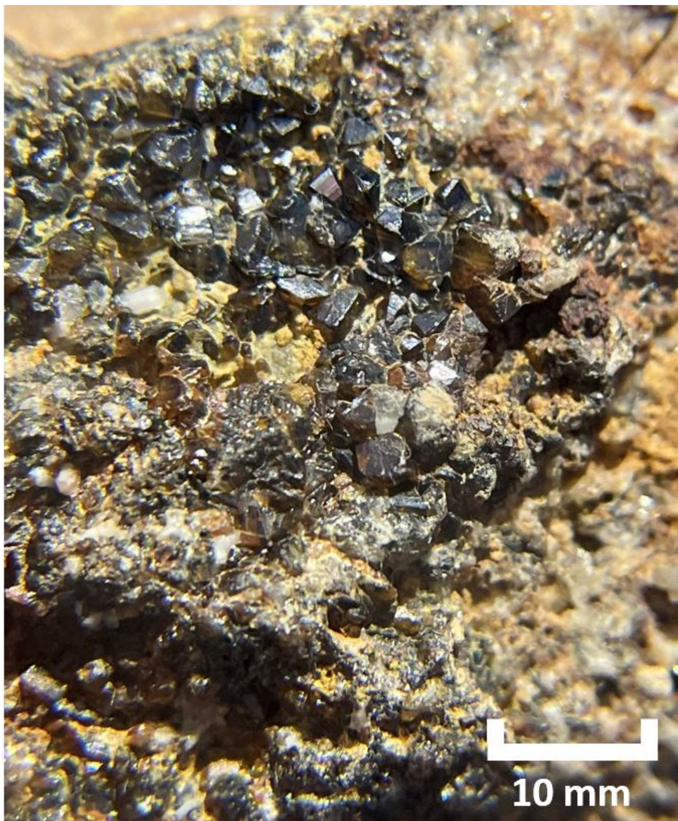
Figure 8. Coarse cassiterite within a fracture in quartzite from La Grana
