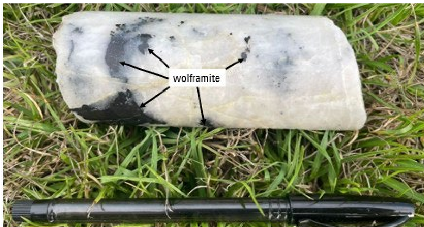
Figure 14. Close-up image of NQ diameter drill core from C2124A from 887.9-888.0m depicting coarse grained wolframite within a steeply dipping cross-cutting quartz vein.
