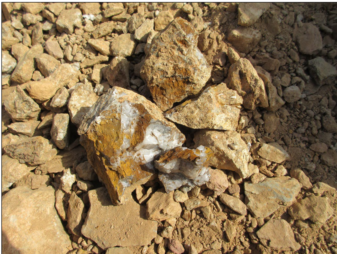
Figure 7: Rock chip sample of quartz veins from spoil pile which returned 79.50g/t Au
