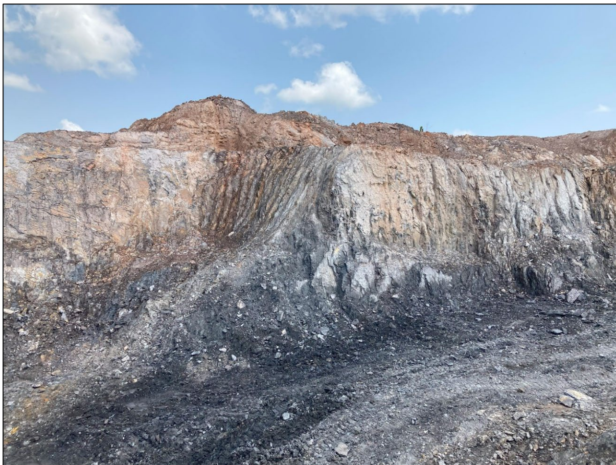
Figure 30: CML's Lauzoua mine in Côte d'Ivoire with sheared vertical manganese bands similar to the sheared manganese on Mako's Korhogo Project such as on outcrop at Anomaly D (refer Figure 27)
