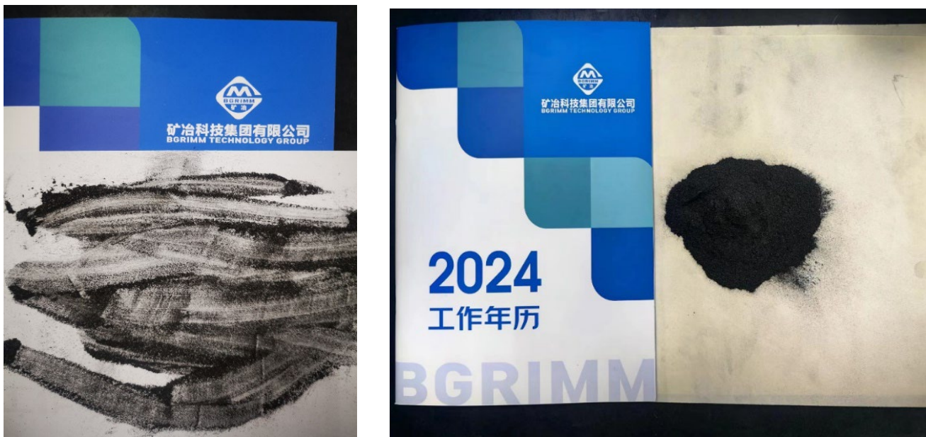
Figure 11: Graphite concentrate produced from the oxide metallurgical samples from the Oar Graphite Project
